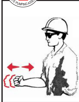
1. START PUMP SPEED UP
