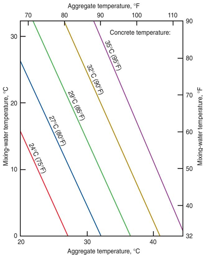
**Fig. 13-5. Temperature of freshly mixed concrete as affected by temperature of its ingredients. Although the chart is based on the following mixture, it is reasonably accurate for other typical mixtures:**
