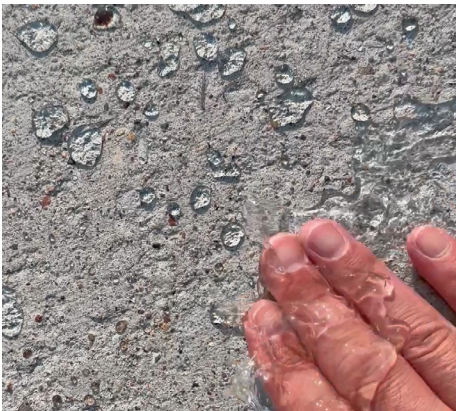
Water beading effect of Siloxane Sealer and Salt Barrier
